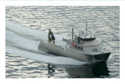
86.7 feet Length Overall 26 feet on the beam 27 knot capability
